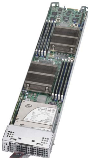
Figure 4-1. MBI-6219G-T Blade Unit Front View
