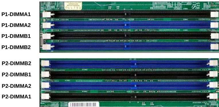
Figure 3-3. 4-slot DIMM Numbering
