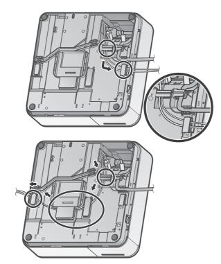
To ensure the main unit is not tilted when installed, beware that cables do not protrude from the hooks while the cables were routed.
