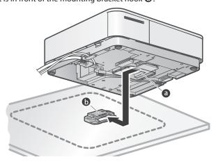
Slide the main unit so that the mounting bracket hook enters the slot to secure the main unit in place.
