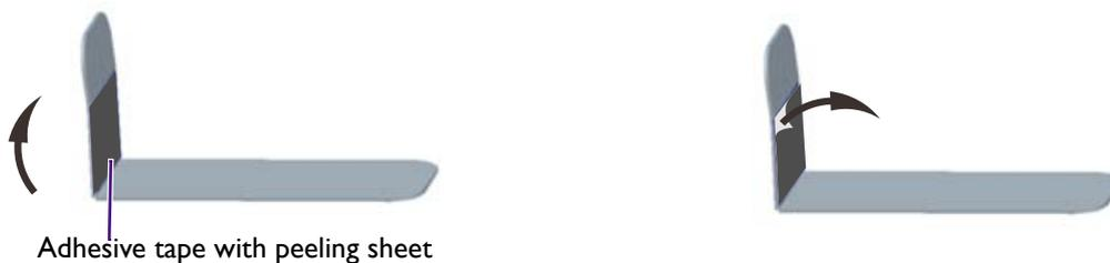
3. Stick the pad to the edge where another display will be stacked as illustrated. Each edge should have 3 gap inspection pads attached.
