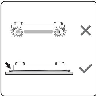
When you want to place the display face down, prepare a flat and horizontal surface that is larger than the display and spread a thick protective sheet on it.
