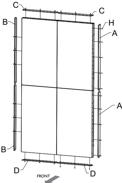
2. On each corner, mount a corner enclosure piece and fasten each one with 4 of the 5mm M3 screws. Where the displays meet, use a flat enclosure piece, and fasten each of these too with 4 of the 5mm M3 screws.
