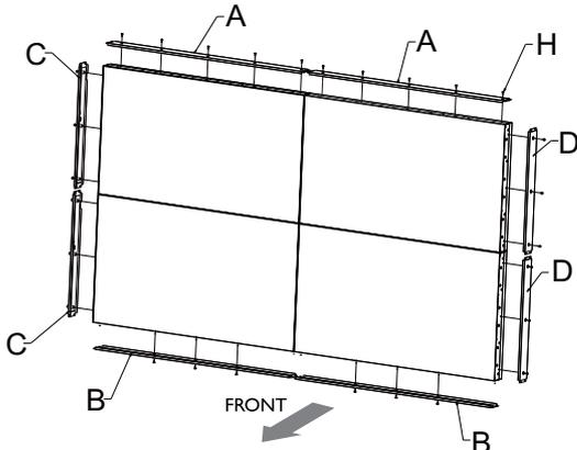
2. On each corner, mount a corner enclosure piece and fasten each one with 4 of the 5mm M3 screws. Where the displays meet, use a flat enclosure piece, and fasten each of these too with 4 of the 5mm M3 screws.
