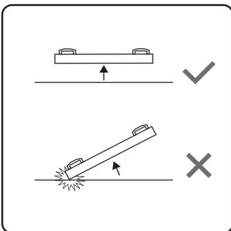
Lift the display up horizontally by holding the four (4) handles. Do not lift the display against its corner.
