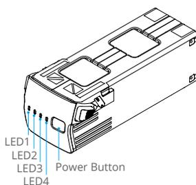
**📖** The battery level LEDs display the power level of the battery during discharging. The statuses of the LEDs are defined below:
