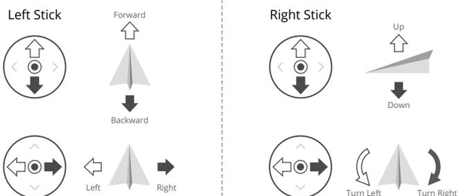
The default control mode of the remote controller is Mode 2. In this manual, Mode 2 is used as an example to illustrate how to use the control sticks.
