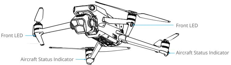
When the aircraft is powered on but the motors are not running, the front LEDs glow solid red to display the orientation of the aircraft.
