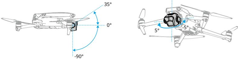
Use the gimbal dial on the remote controller to control the tilt of the camera. Alternatively, do so through the camera view in DJI Fly. Press and hold the screen until the camera adjustment bar appears. Drag the bar up or down to control the tilt and left or right to control the pan.
