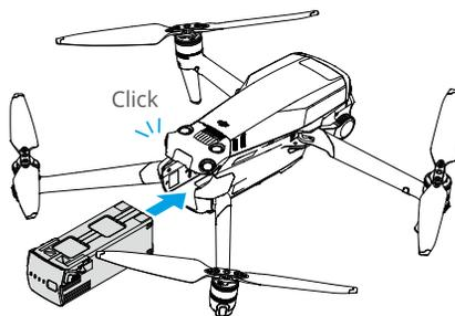
Press and hold the textured part of the battery buckles on the sides of the battery to remove it from the compartment.
