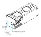
The battery level LEDs display the power level of the battery during discharging. The statuses of the LEDs are defined below:
