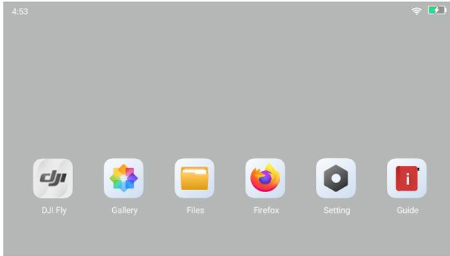
The top of the touchscreen displays the time, Wi-Fi signal, and battery level of the remote controller.
