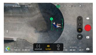
b. Tap on the bottom of the screen to switch to Point of Interest. After setting the direction and speed, tap GO to start flying.
