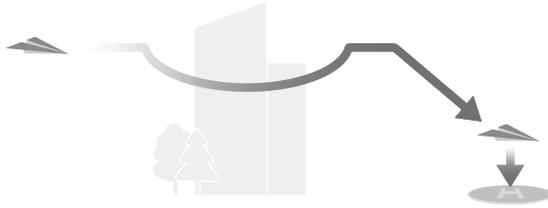
2. **Preset:** if the aircraft is further than 50 m from the Home Point when RTH begins, the aircraft will plan the RTH path, fly to an open area while avoiding obstacles, ascend to the RTH Altitude, and return to home using the best path.
