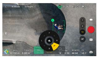
Tap the shutter/record button to take photos or start recording. View the footage in Playback ▶ .
