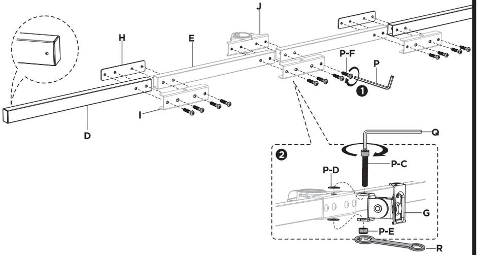
Attach the sliding parts (F) to both sides of the arm.
