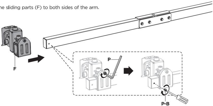
Keep the arm parallel to the edge of the table when attaching it to the pole.
