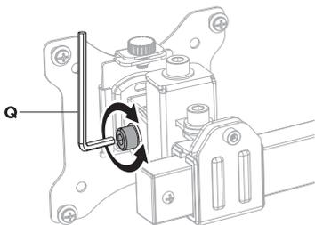
**Note:** If the display does not stop at your desired position, tighten the screws as shown.
