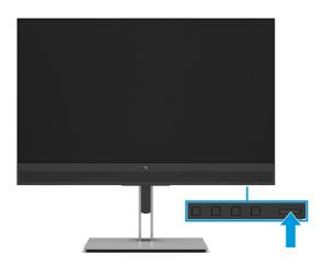
When you first turn on your monitor, a monitor status message is displayed for 5 seconds. The message shows which input is the current active signal, the status of the auto-switch source setting (On or Off; default setting is On), the current preset display resolution, and the recommended preset display resolution.
