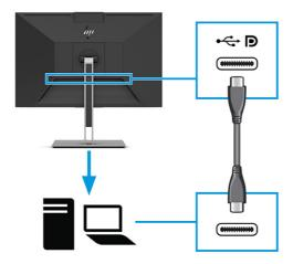
NOTE: The monitor's USB Type-C port provides network, data, video, and power delivery (up to 65 W).
