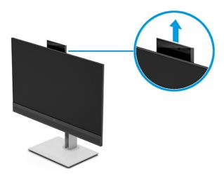
NOTE: If a camera firmware update is required, the camera must be in the unlocked position while updating the firmware.
