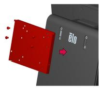
Attach the other bracket to the AiO system or monitor using the 4 M4 screws included in the kit.
