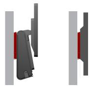
Hang the AiO on the wall bracket and secure using 2 M3 screws included with the kit on the left and right side of the bracket.
