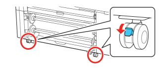
Secure the two adjustable feet on the back of the printer.
