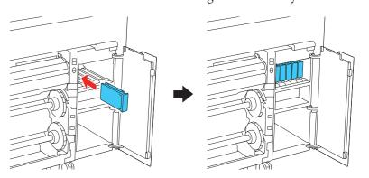
**Note:** Make sure all of the ink cartridges are properly inserted in the product; otherwise printing is not possible.
