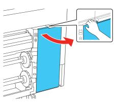
Insert the cartridges in the slot for each color as described on the label inside the ink cover. Push the cartridges in until they click.
