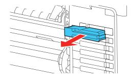
Insert the ink pack into the tray with the color label facing up and push it down as shown.
