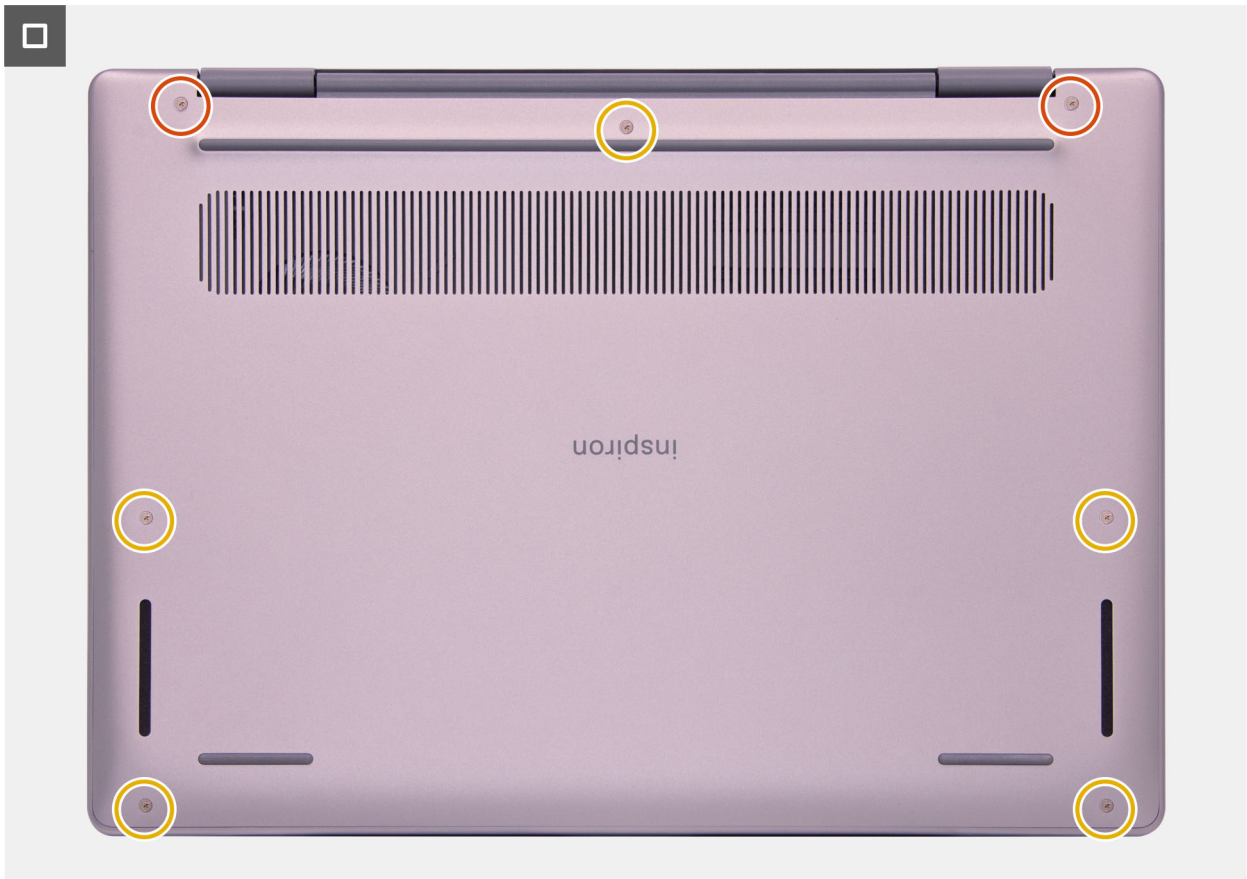
Figure 15. Installing the screws
