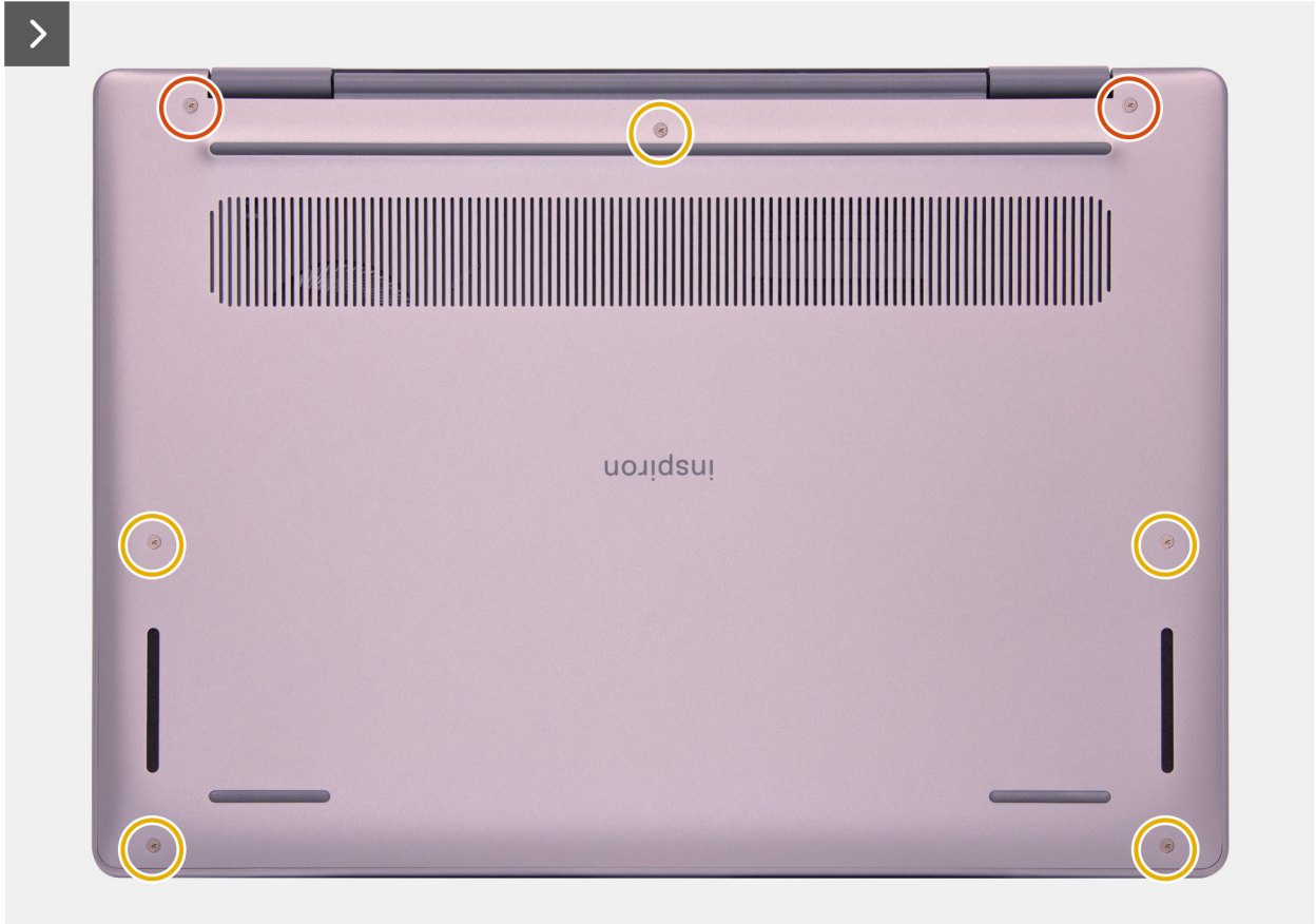
Figure 10. Removing the screws
