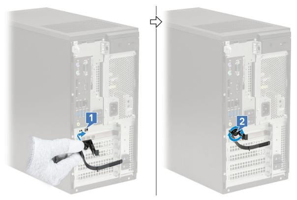
Route the cables through the slot of the cable cover [1], and connect them to their respective ports on the system [2]. Secure the cable with the cable tie and lock the tab in place [3].
