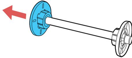
3. Insert the spindle into the roll paper core so that the end of the roll paper is facing towards you.
