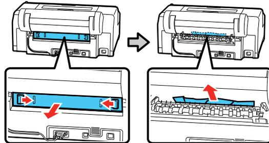
4. Replace the rear unit. Push it into the printer firmly until you hear a click.
