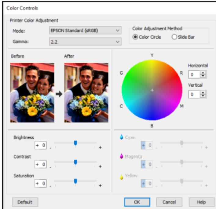
The Color Controls screen lets you specify values for adjusting brightness, contrast, saturation, and individual Cyan, Magenta, and Yellow color tones. You can choose from two Printer Color Adjustment modes and two Gamma settings, and use either a color circle or slide bar to adjust color.
