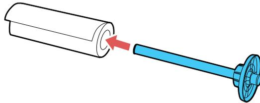
4. Press the roll paper against the fixed paper stop until that there is no gap between the paper stop and the roll paper.
