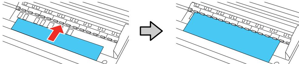
7. Align the edge of the paper with the guide line on the output tray.
