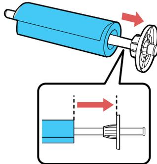
5. Insert the black paper stop onto the spindle and press in until there is no gap between the paper stop and the roll paper.
