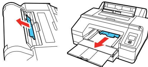
2. Open the printer cover. Remove any other jammed paper as necessary.
