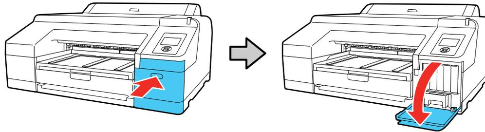
2. Use the handle on the bottom of the maintenance tank to carefully pull it out of the product without tilting the tank.
