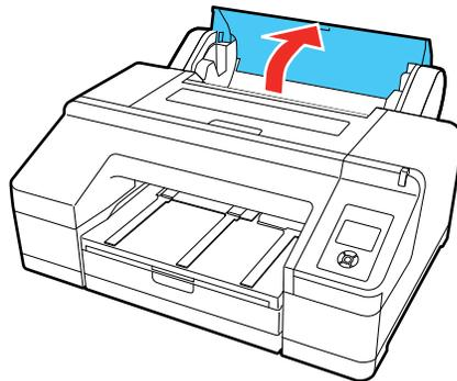
5. Place the roll paper in the printer as shown (the black end of the spindle goes on the left).
