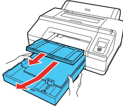
2. Remove any jammed paper from the front of the printer.
