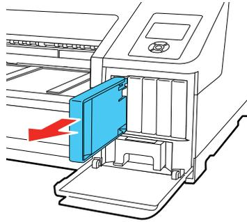
**Note:** Dispose of used cartridges carefully. Do not take the used cartridge apart or try to refill it.
