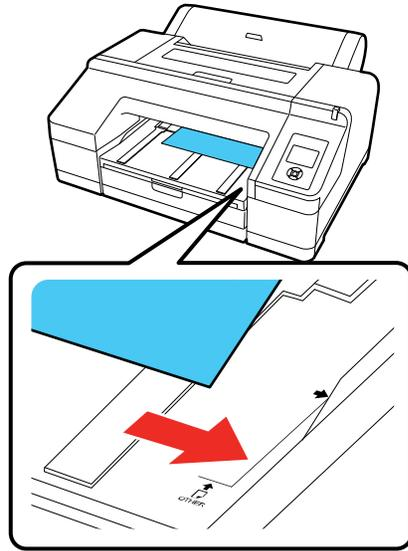
8. Press the
