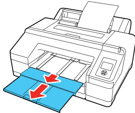
8. Press the
