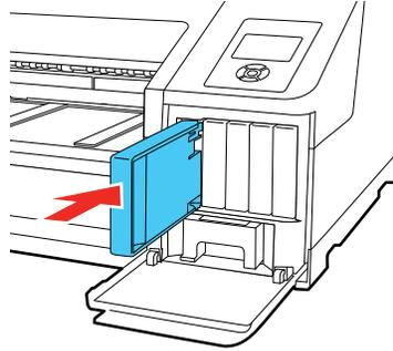
**Caution:** Do not remove and re-insert cartridges more often than necessary. Doing so can break the needle valve seal and allow air to enter the ink tubes, damaging the nozzles.
