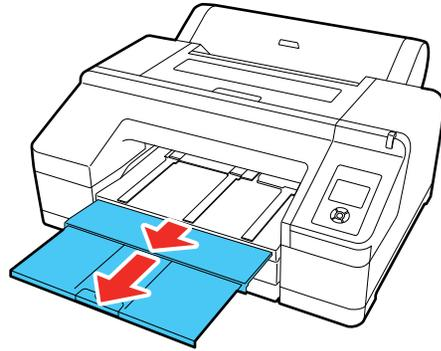
**Note:** If you are printing on plain paper or thin media types, or if you are using the optional Spectroproofer, raise the paper eject support. This prevents paper from curling up in the output tray, which can cause paper jams and print head strikes.
