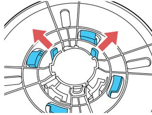
3. To remove the gray adapter from the other paper stop, slide it off the spindle.
