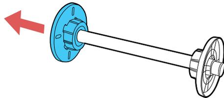
2. Slide the spacer all the way onto the spindle until it reaches the gray paper stop on the other end. Make sure the holes in the spacer and paper stop line up exactly.
