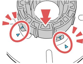
3. Insert the other gray adapter onto the spindle and attach it to the other paper stop.
