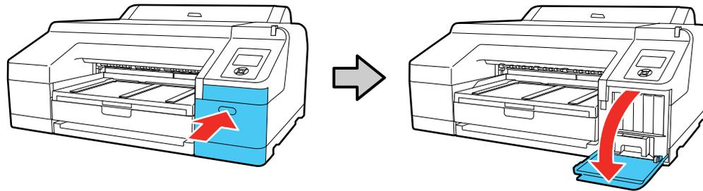
3. Press in on the ink cartridge you want to replace. The ink cartridge pops out slightly.
