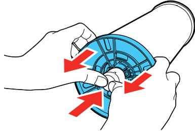
5. Remove the roll paper from the spindle.
