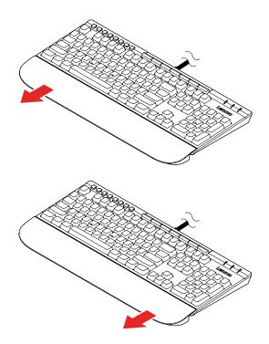
Attention: Do not apply excessive force in other directions to avoid damage.
