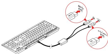
Note: It is recommended that you connect both cables of the keyboard to your computer as shown above to ensure the full function of the keyboard.
