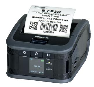
The B-FP3D comes with a full colour graphical LCD display for ease-of-use and enhanced efficiency.
