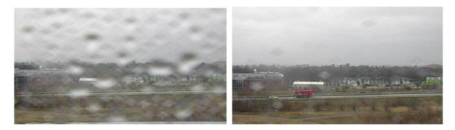
Snapshot from a camera's live view before and after speed dry has been activated.
