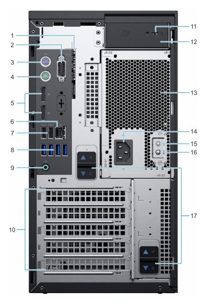
Figure 2. Rear view of the system
