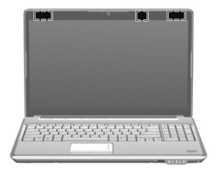
NOTE: For optimal transmission, keep the areas immediately around the antennas free from obstructions.
