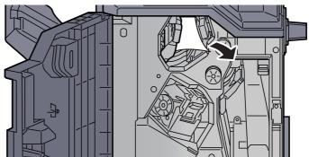
Q Return the conveyor guide (D4) to the original position.
