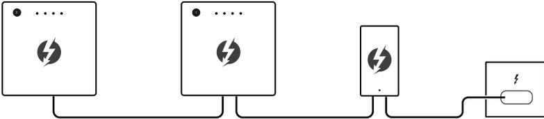
You can also daisy-chain monitors on the front IO panel. Please note that monitors should be the last devices on the chain.
