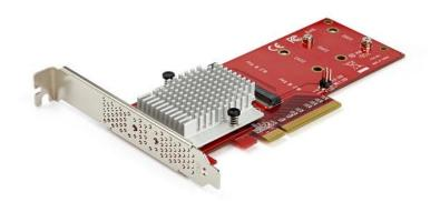
Upgrade your system speed and performance with this Dual M.2 PCIe SSD Adapter. It lets you add two high performance, enterprise-class PCIe 3.0 M.2 SSDs (NVMe and AHCI) into the PCIe 8-lane or larger slot of your desktop workstation or server.
