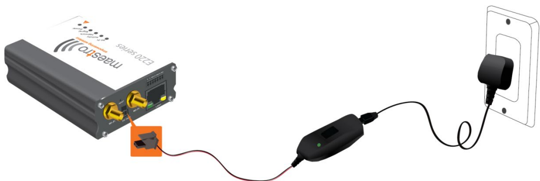
Figure 9: Connecting the AC power connector
