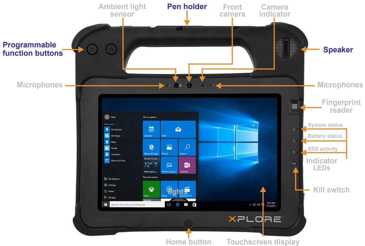
The XPAD tablet has the speaker, a pen holder, and programmable function buttons in the handle.
