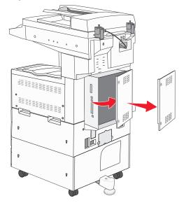
Use the illustration to locate the connector for the option you want to install.
