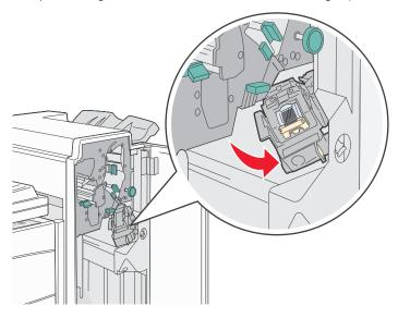
**3** Firmly pull the colored tab to remove the staple cartridge.
