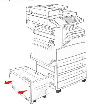
3 Raise the top door, and lift the jam access cover.
