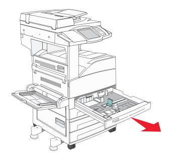
2 Squeeze the side guide tab, and slide the guide to the outside of the tray.
