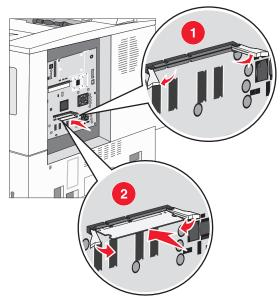
6 Make sure each latch fits over the notch on the end of the card.
