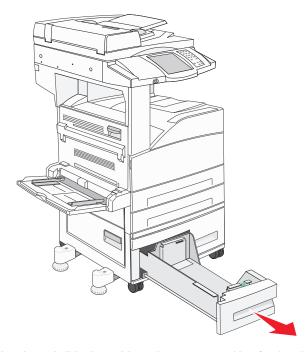
2 Squeeze the front guide tab, and slide the guide to the correct position for the size media you are loading.
