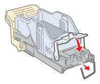
8 Push the cartridge holder firmly into the stapler until the holder *clicks* into place.
