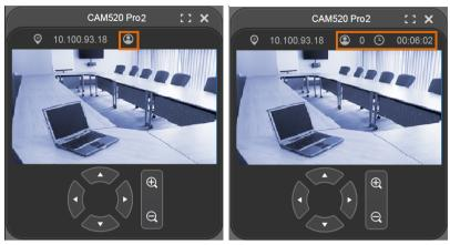
Control Panel: To control the camera direction, zoom in and out, and to enable/disable the "Smart Framing" during your video call.
