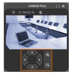
Setting: Click "Setting" button to setup parameters of the camera and speakerphone. Click arrow icon to leave the Setting page.
