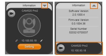
8. **Camera:** Click the camera icon to view the camera live view. IP address is displayed as well. Click the X icon to close the camera live view. If the live video did not appear, please check the camera and the laptop/PC connection to make sure all are correct and well connected.
