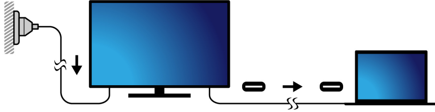
Figure 2. A connected display supplies power to the PC through the Power Delivery-compliant USB Type-C connector
