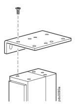
2. Install the Rack PDU on a vertical mounting rail in your rack or enclosure.
