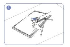
Lift and remove the stand in the direction of the arrow as shown in the figure.
