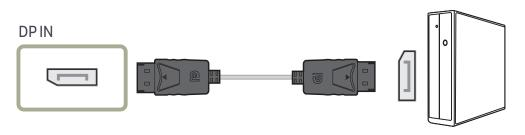
To display 3840 x 2160 @ 60 Hz, use a DP cable that supports 3840 x 2160 @ 60 Hz. Make sure that the graphics card of the DP source supports 3840 x 2160 @ 60 Hz.
