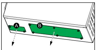
3. Drill or punch holes for cables or conduits in the gland plates for signal cables (A) and power cables (B).
