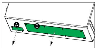
3. Drill or punch holes for cables or conduits in the gland plates for signal cables (A) and power cables (B).
