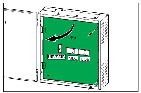
2. Measure and mark the four mounting hole locations on the wall.
