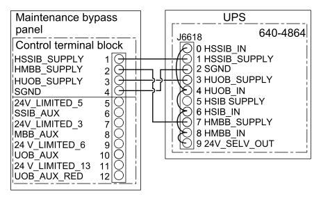
2. Connect the non-Class 2/non-SELV signal cables from the control terminal block in the maintenance bypass panel to the UPS as per your configuration.
