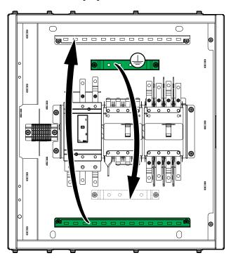
2. Remove the gland plates in the top or bottom of the maintenance bypass panel.
