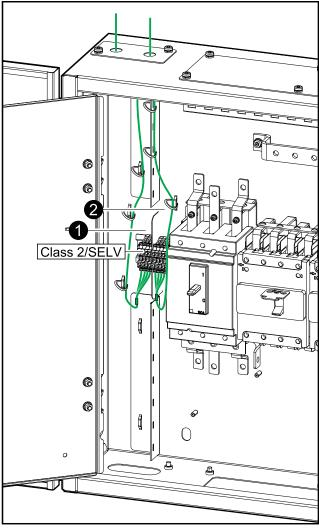
1. Connect the Class 2/SELV signal cables for the breaker indicator lights from the control terminal block in the maintenance bypass panel to the UPS as per your configuration.
