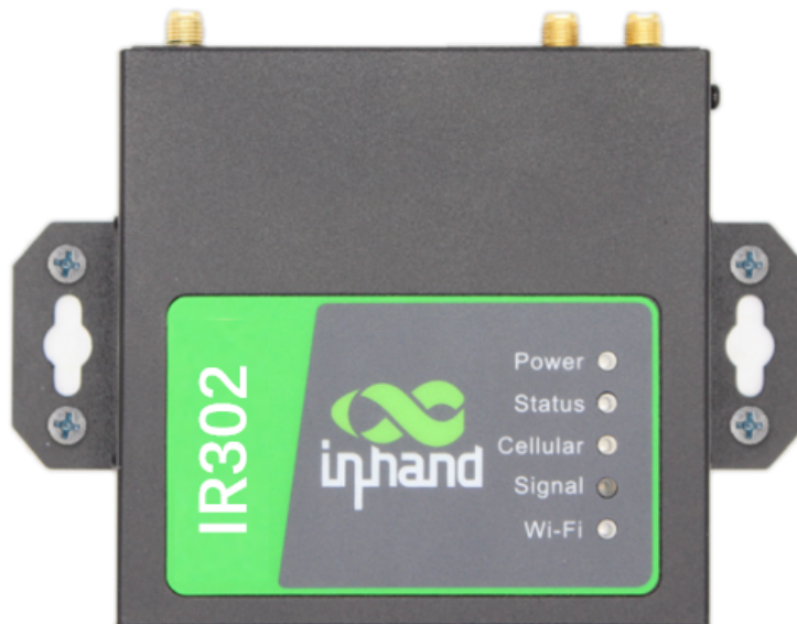
Fig. 4-2-1 Wall Hanging Installation
