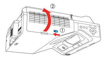
3. Pull the air filter out of the projector.
