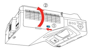
3. Pull the air filter out of the projector.
