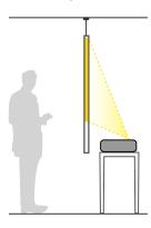
Wherever you set up the projector, make sure to position it squarely in front of the screen, not at an angle.
