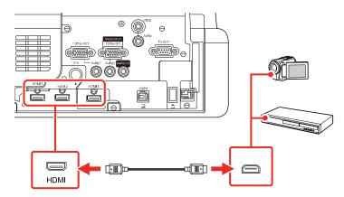
**Note:** The projector converts the digital audio signal sent from your video source into a mono analog signal for the internal speaker or a stereo analog signal if you are connecting to external speakers.
