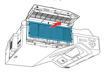
4. Vacuum the front of the air filter (the side with the tabs) to remove any remaining dust.
