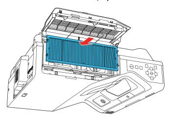
5. Close the air filter cover and slide the latch.
