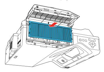
6. Close the air filter cover and slide the latch.
