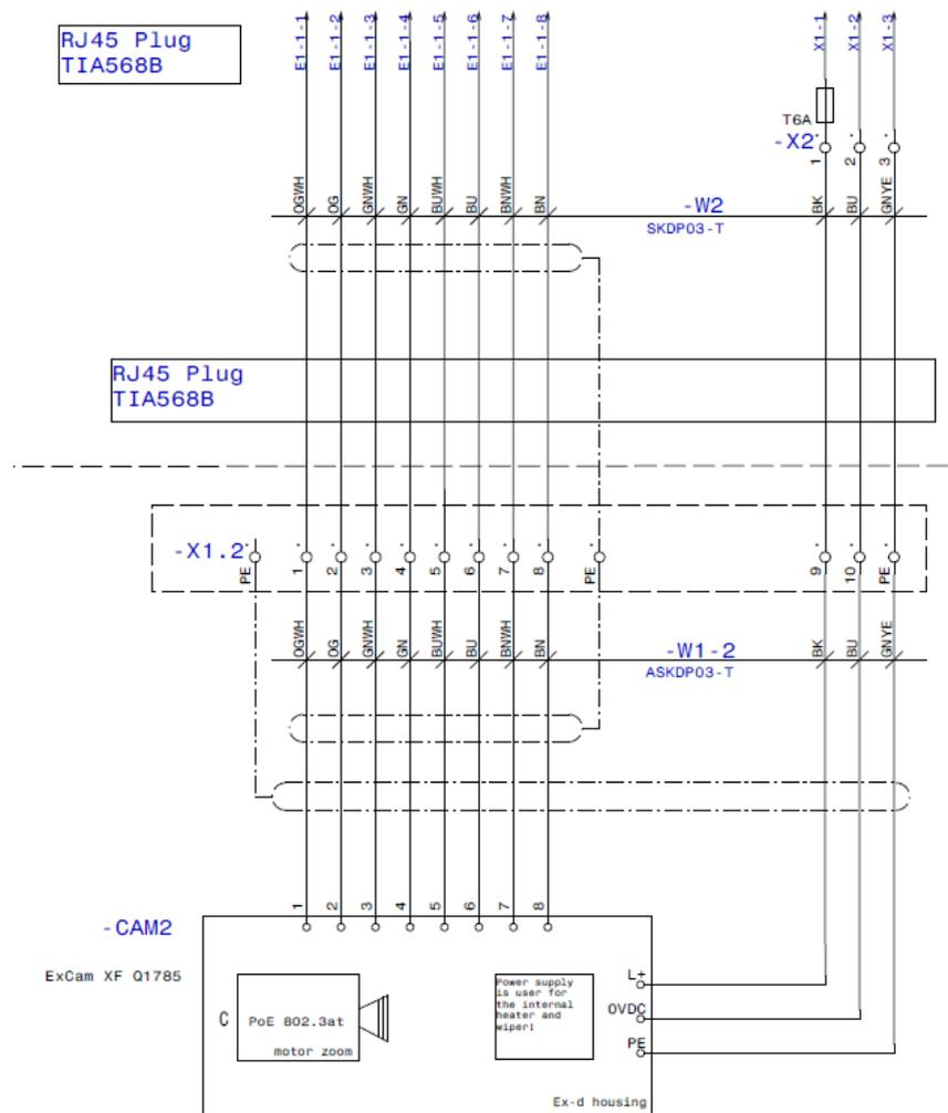
Fig. 5-4 Sample circuit of terminal box ExtTB-3
