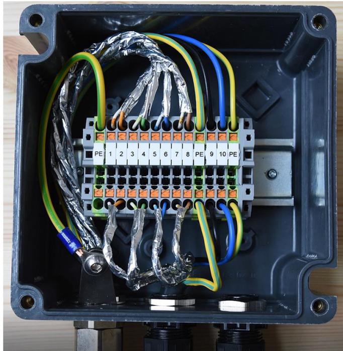
Fig. 5-5 Photo of the occupied terminal box ExTB-3
