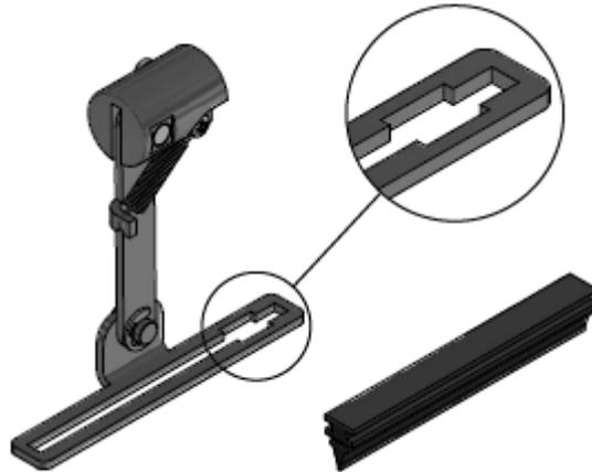
Fig. 8-1. How to replace the wiper lip
