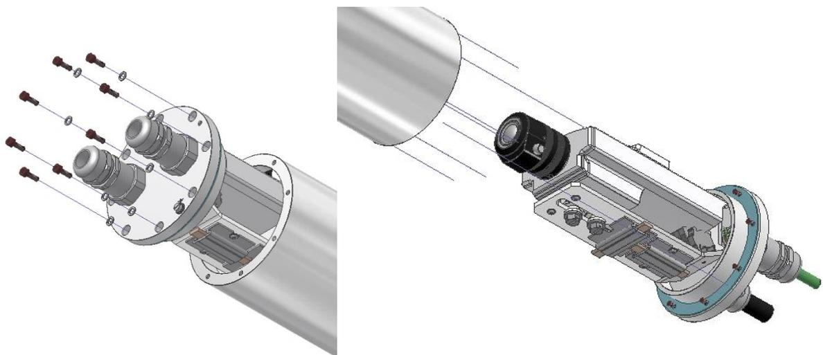
Fig. 6-3 Opening the ExCam XF Q1785 (similar illustration)
