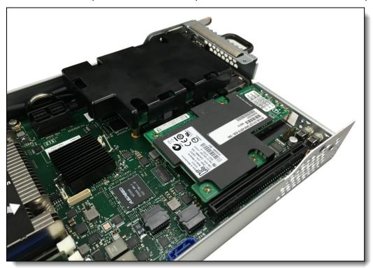
Figure 10. Adapters installed in the sd350
