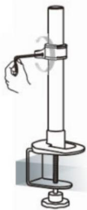
2. Slide the Monitor Mount (2) onto the Support Post (1) until it rests on the Collar (7) and tighten the set screw using the M3 Allen Wrench (15).
