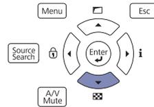
2. Press the **Enter** button to change the test pattern.
