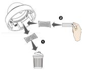
15. Ensure the inside of the dome cover is free of dust and particles by gently wiping the inside with a clean lint free cloth or blowing the dust away. Install the dome cover and remove the protective wrap.
