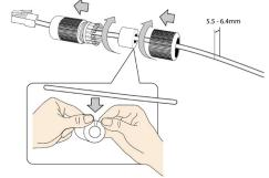
6. Connect the Ethernet cable. The cable can be stored in the EMT tubing or in the hole in the wall or ceiling.
