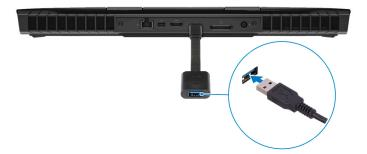
8 Connect the Oculus Rift tracker for Touch to the USB Type-A port on the dongle.
