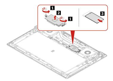
Step 2. Install the M.2 solid-state drive and M.2 solid-state drive bracket in reverse order.
