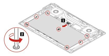
b. Remove the battery as shown below.
