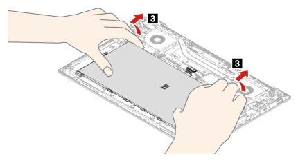
Step 2. Install the built-in battery in reverse order.
