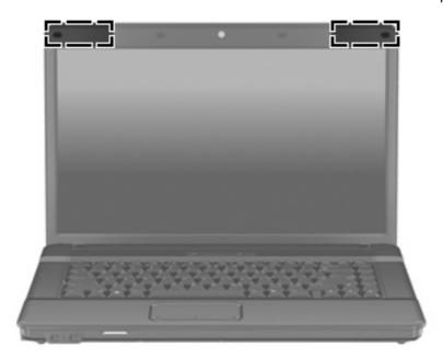
NOTE: For optimal transmission, keep the areas immediately around the antennas free from obstructions.
