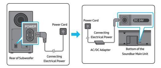
Make sure to rest the AC/DC Adapter flat on a table or the floor. If you place the AC/DC Adapter so
