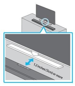
As illustrated in the image, align the center of the Soundbar with the center of the TV, carefully place the Soundbar onto the TV stand. For optimal sound quality, position the Soundbar at least 1.2 inches (3 cm) away from the TV front.
