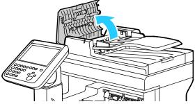
3. If the paper is jammed in the exit of the duplex automatic document feeder, pull it out as illustrated.
