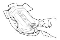
3. Push the USB wireless dongle down to release it from the compartment.
