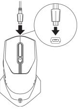
**2.** Connect the other end of the USB wireless dongle extension/charging cable to the USB port on your desktop or laptop.
