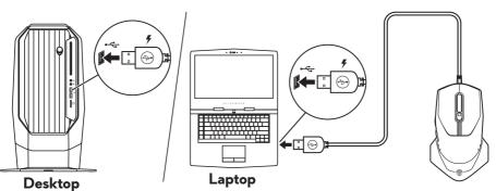
**3.** Wait until the battery indicator turns solid green. Solid green color indicates that the battery is fully charged.
