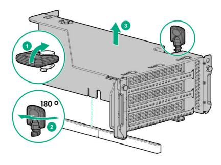
For secondary bays, remove the rear wall blank.
