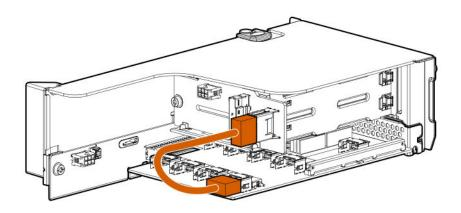
Rear 2SFF drive option in the secondary slot to a SAS Expander in primary slot
