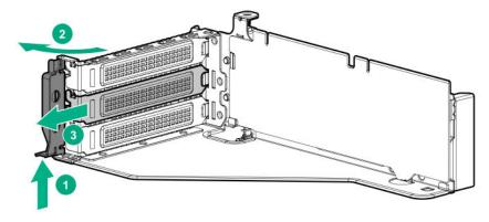
13. Install the GPU into the riser.
