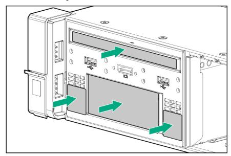
• If a 2SFF drive cage is installed, then install the airflow labels as shown.
