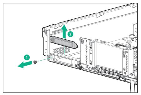
7. Install the FlexibleLOM adapter:
