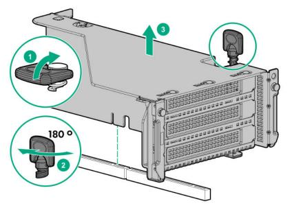
Remove the rear wall blank.
