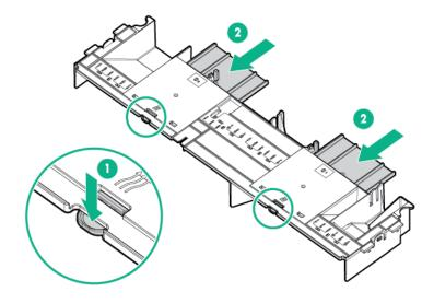
8. Install the appropriate retention clip onto the air baffle. Primary, secondary, and tertiary positions are shown. Install the clip that supports your configuration.
