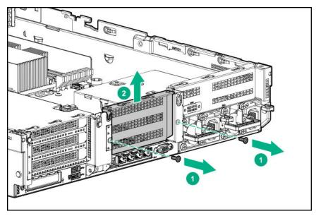
12. Remove the PCIe blank.
