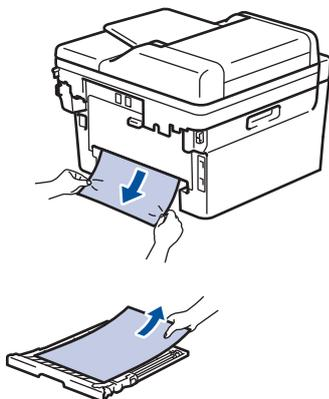
5. Remove paper that may have jammed under the machine due to static electricity.
