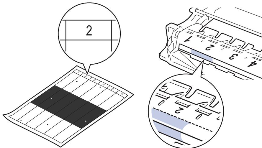
10. Rotate the wheel at the end of the drum unit while pushing the shaded part, as shown in the illustration, to find the mark or foreign material.
