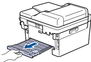
4. Pull the jammed paper out of the machine or out of the 2-sided tray.
