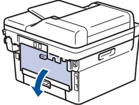
3. Pull the blue tabs at the left and right sides toward you to release the fuser cover.
