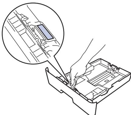
5. Wipe the two pick-up rollers inside the machine to remove dust.
