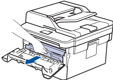
4. Push down the green lock lever, and then take the toner cartridge out of the drum unit as shown in the illustration.
