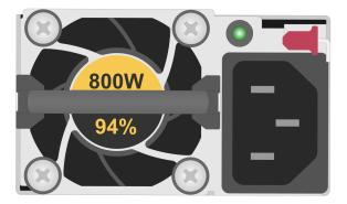
Each power supply has a status LED that indicates whether power is present or whether a power fault has occurred. The status LED is located to the left of the red latch lever.
