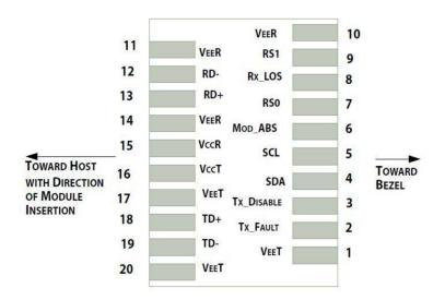
Pin-out of connector Block on Host board
