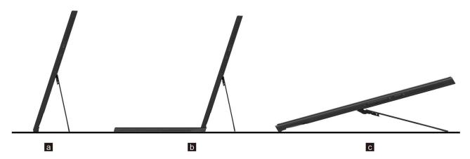
The kickstand is multi-positional. You can adjust the kickstand to various angles for a comfortable user experience.
