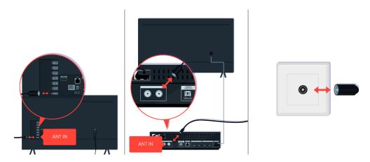
Check the antenna and input cable connections.
