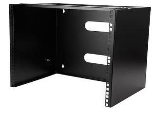
This wall-mount bracket provides 8U of space for mounting shallow rack-mount equipment that's 13.75 in. (34.93 cm) deep or less to the wall, such as patch panels or network switches.
