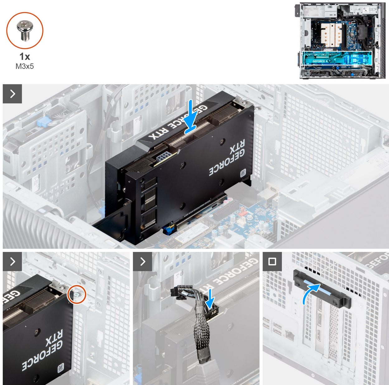
Figure 40. Installing the powered graphics card
