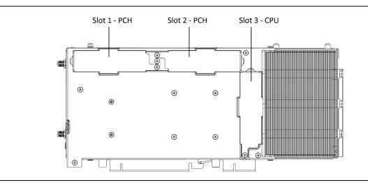
Figure 4. Location of NUC 13 Extreme Compute Element M.2 Slots
