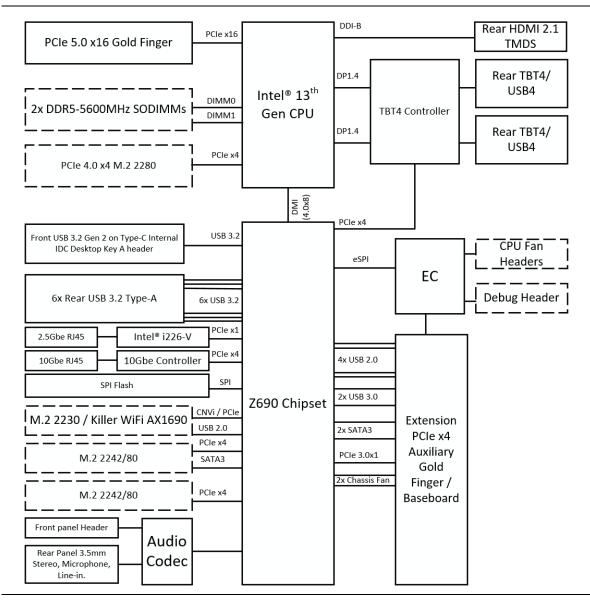
Figure 1. Block Diagram – NUC 13 Extreme Compute Element
