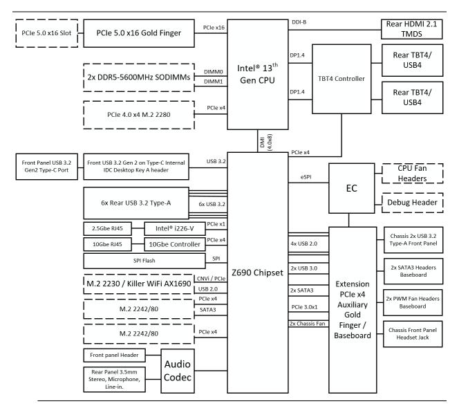
Figure 2 is a block diagram of the major functional areas of the Intel<sup>®</sup> NUC 13 Extreme Kit.
