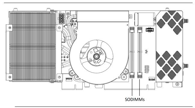
Figure 3. SODIMM Location on NUC 13 Extreme Element
