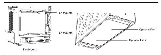
Figure 19. Optional Chassis Fan Mounting Locations
