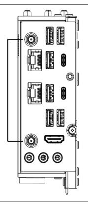
Figure 13. Location of the Antenna Connectors
