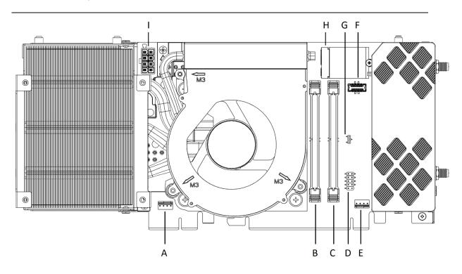
Figure 12. NUC 13 Extreme Compute Element Headers and Connectors
