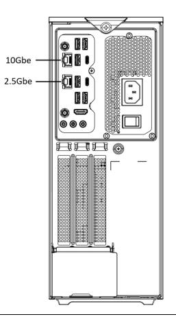
Figure 5. NUC 13 Extreme Kit LAN Controller Layout
