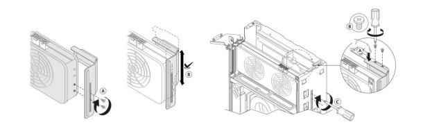
Figure 18. GPU support Bracket Installation Guidance
