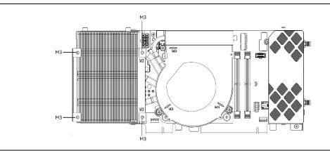
Figure 20. Optional NUC Element Fan Mounting Location
