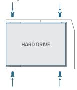
4. Insert and screw the bracket back to the HomeBase, then put the top lid back into place.
